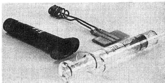
Photo 3. Coil construction: an original hypodermic syringe together with the finished body and the pc "T" piece and coil prior to final assembly
